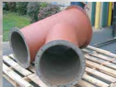
Steel mill - sinter dust extractor ducting
